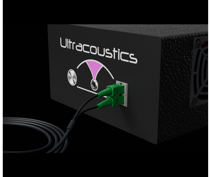
Fully seated: both optical connections are made together.
